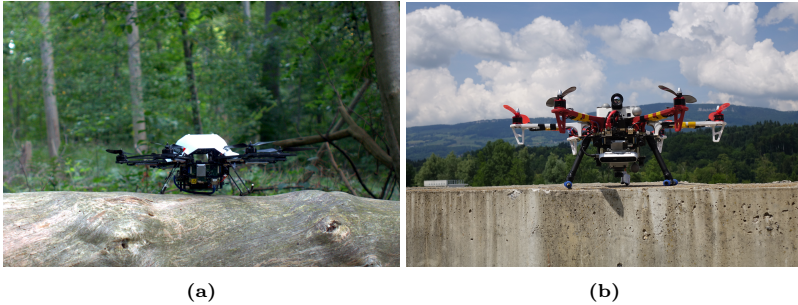
Figure 1.2: Two of the MAV systems used for this thesis, including various sensor configurations. (a) is an Asctec Firefly, with a dual-core 1.7 GHz i7 CPU and a stereo VI Sensor [78] as the only perception. (b) is a custom-built system based on the DJI FlameWheel F550 frame, with an Intel NUC on-board, and outfitted with a VI Sensor, an Intel D400 RGB-D sensor, a thermal camera, and a higher-resolution downward-facing camera.
