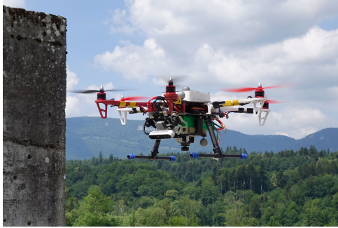
Figure 9.1: The platform used for collecting the test datasets, a custom-built drone using the DJI FlameWheel F550 frame, an Intel NUC for on-board processing, Pixhawk for flight control, VI Sensor for monocular state estimation and stereo depth, and an Intel RealSense D415 for RGB-D input.
