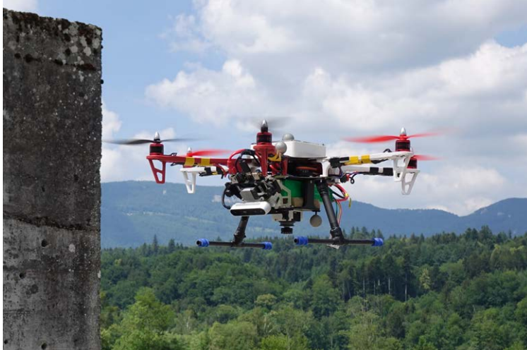
Figure 1: The platform used for collecting the test datasets, a custom-built drone using the DJI FlameWheel F550 frame, an Intel NUC for on-board processing, Pixhawk for flight control, VI Sensor for monocular state estimation and stereo depth, and an Intel Realsense D415 for RGB-D input.
